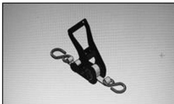
**Figure 3:** The Ratchet used in pulling the pipe.
