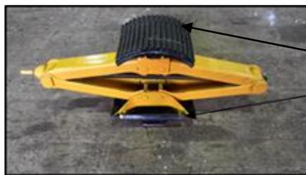
Reinforced rubber strips for optimum gripping on upper and lower jaw.
