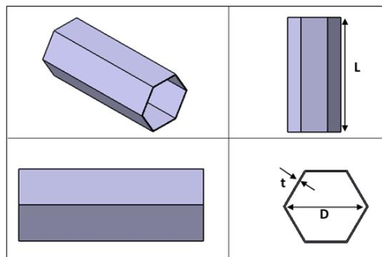
Figure 5: Single-cell Crash-box geometry using ANSYS/Design Modeler Geometry
