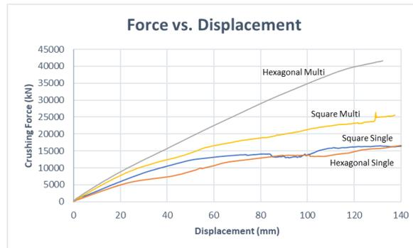
Figure 10: Crushing forces created by time consumption during impact.
