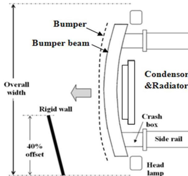
Figure 3: Layout of Frontal Crash Management System with Engine, Condenser and Electrical System, (Kiran Cheni, Sinha, & Narayan, 2013)
