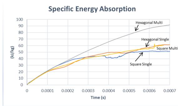
Figure 9: Specific Energy Absorption (SEA) for all four proposed design.
