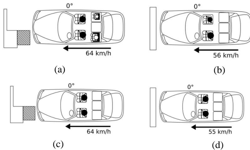
Figure 4: Low-velocity frontal test, (a) NCAP Europe front offset test, (b) NCAP USA front test, (c) NCAP Japan front offset test, (d) NCAP Japan front test, (Crash Tests 2015)
