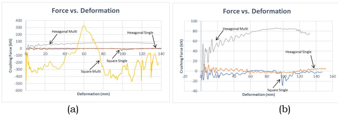
Figure 8: Forces created by energy absorption along the deformation.
