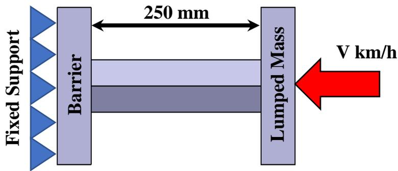
Figure 7: FE Model and loading condition
