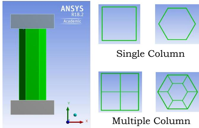
Figure 6: Multi-cell column Crash box cross-sectional view ANSYS/SpaceClaim
