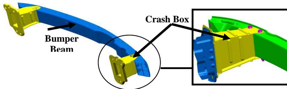
Figure 2: Crash Management System (CMS), Bumper beam and crash box, (European Aluminium Association, 2013b)
