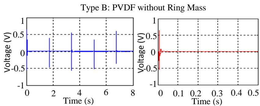
Figure 6(b). Vibration Pattern Of PvdF Without Ring Mass
