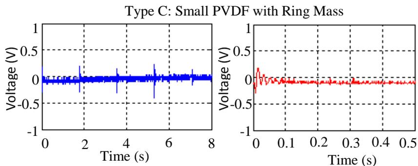
Figure 6(c). Vibration Pattern Of Small PvdF With Ring Mass
