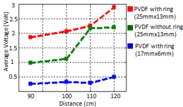
Figure 8. Average Voltage Generated From Different PvdF
