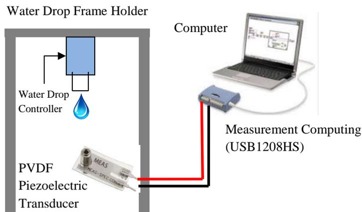
Figure 4. Piezoelectric Energy Harvesters Experiment Setup
