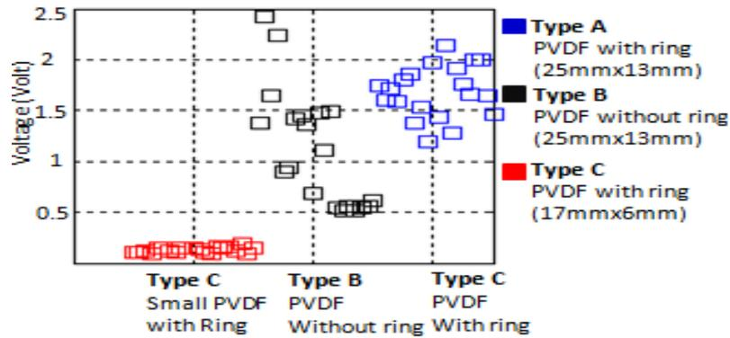
Figure 7. Average Voltage Samples At 90 Cm Height
