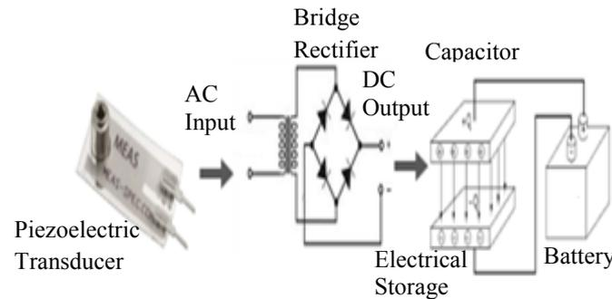
Figure 1. Piezoelectric Energy Harvester System
