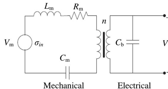
Figure 2. Circuit Representations Of Mechanical And Electrical Portions
