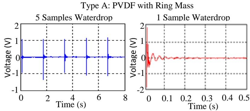
Figure 6(a). Vibration Pattern Of PvdF With Ring Mass
