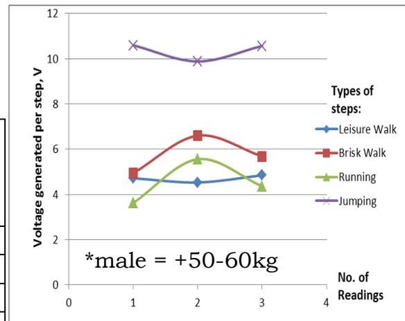
Figure 4.1: Voltage readings per different types of steps.
