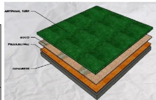
Figure 4.2: Piezoelectric Stepping stone Prototype
